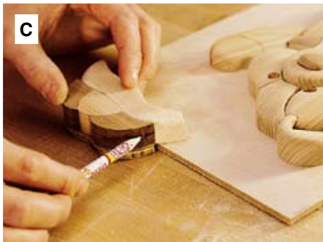
Check the transition between adjacent parts as you contour them. Re-mark and continue sanding as necessary.
