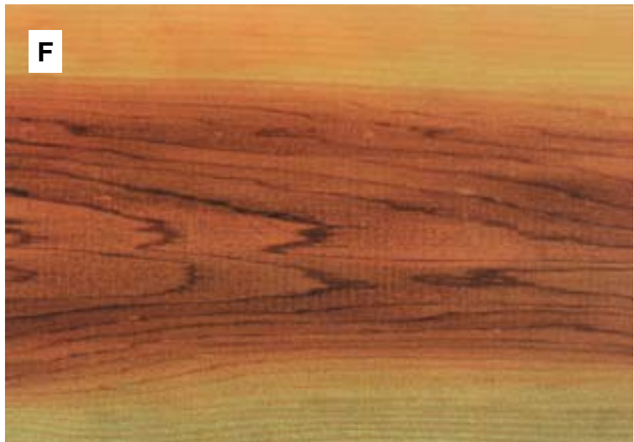
Though it is hard to find, red cedar sap wood can be used as white-colored wood in place of the more common basswood, pine or aspen.
