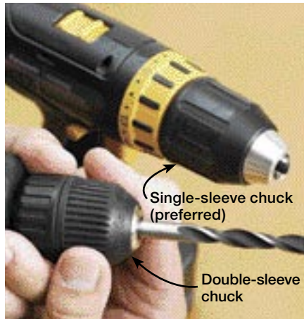
A single-sleeve chuck tightens with only one hand. A double-sleeve chuck requires two hands in close proximity, resulting in a chuck that's "finger tight" rather than "hand tight."
