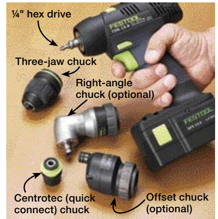
Four different add-on chucks—two standard equipment and two optional—make this drill/driver a versatile switch-hitter in your shop. With none of the chucks mounted, the 1/4" hex drive accepts standard quick-release bits and makes the drill barely longer than its battery pack.
