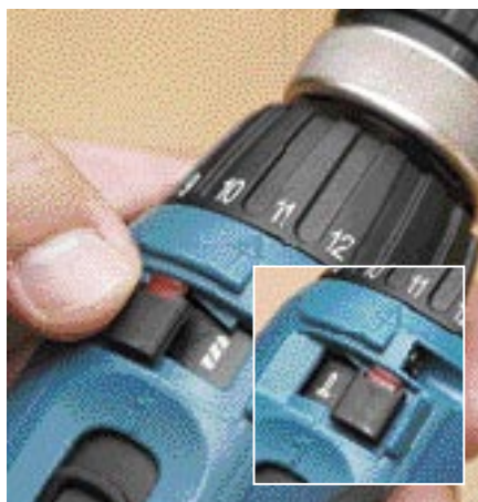
This drill features a switch that disables the clutch in "drill" mode (above) for full-on power. Flipping to "drive" mode (inset), re-engages the clutch.
