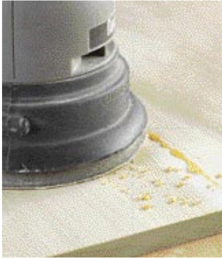
Glue globs can scratch the surface of your work either when they break loose or become trapped on your sanding pad.
