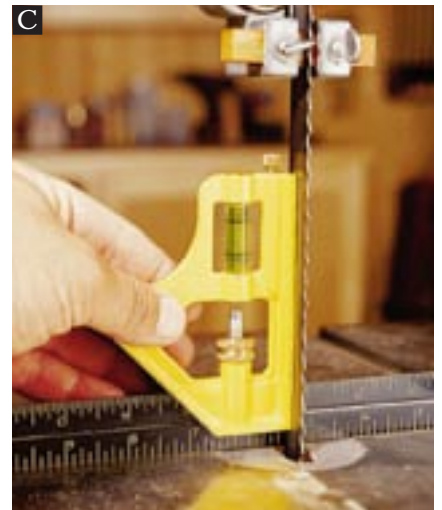
C With the bandsaw table's 0° stop set precisely, you're ready to begin cutting.
