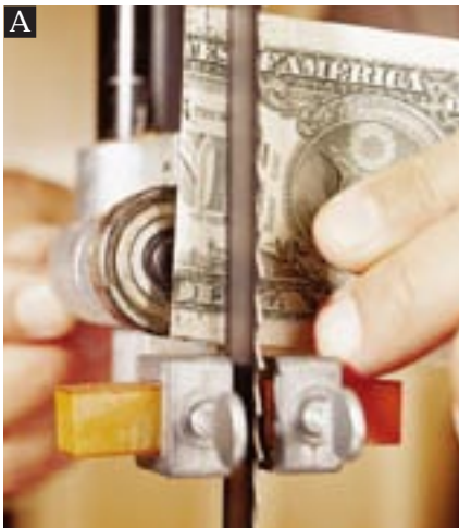
A A double thickness of paper currency provides proper clearance between the thrust bearing and the back edge of the blade.
