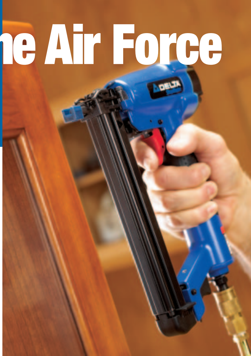
A narrow-crown stapler is the ideal way to effortlessly install a 1/4" plywood back.
